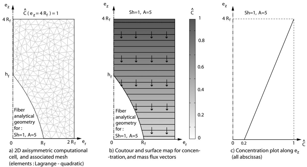
Fig. 4. Numerical validation of the vertical flux hypothesis.
